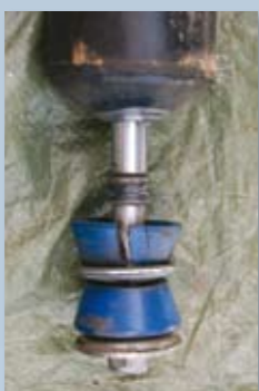
Above: Bodes by the Land Rover dealership in Stavrapol led to this – bushes fitted in the wrong place, with some parts missing altogether.
