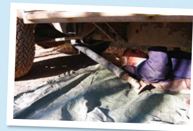
Above Paul removes the propshaft, which relieves the strain on the transfer box and reduces the clunking and grinding sounds. Below Setting up camp in Siberia for the first night.
